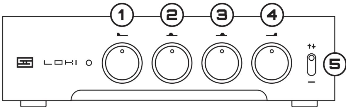
**1 Bass Adjustment.** (20Hz) Turning the knob clockwise increases bass, turning it counterclockwise decreases bass. Like all the adjustments on Loki, it has a gradual effect when first turned off of the center position, for subtle adjustments.
