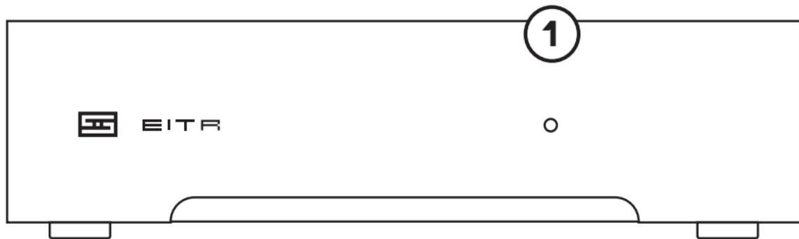
**1 Power Light.** When the power is switched on, this light will illuminate.
