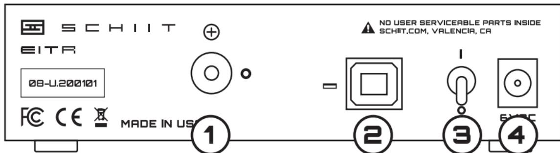
**1 Coaxial SPDIF Digital Output.** Connect this to your DAC with a high-quality cable. If you'd like, you can even use a fancy "75 ohm" version, though this doesn't make a huge difference in performance, unless you're using some unshielded, hand-braided thing that's inappropriate to digital.
