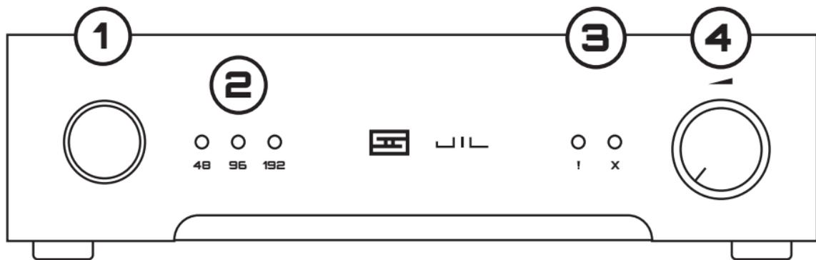
**1 Sample Rate Selector.** Press to step between three different sample rates—48kHz, 96kHz, or 192kHz. Jil does not do 44.1kHz multiples.
