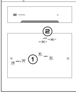
There are no controls on the front, just a LED. When the light is on, it's on. Flip Mani over and you'll see a bunch of switches.
