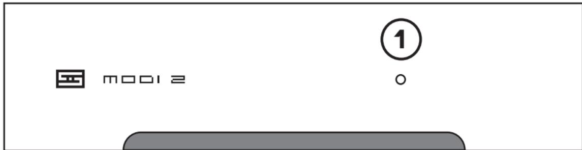
**1** When the light is on, that means Modi is powered up. That'll happen every time it's plugged into an active USB port. Leaving it on all the time is fine.
