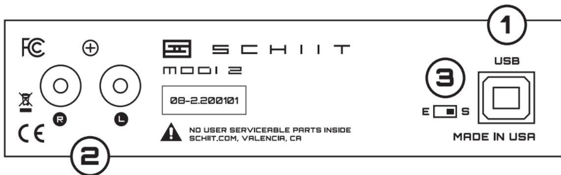
**1** Connect your source (usually a computer) to the Modi 2's USB input, helpfully labeled "USB." Use a short, truly USB 2.0-rated cable (2 meters or less.)
