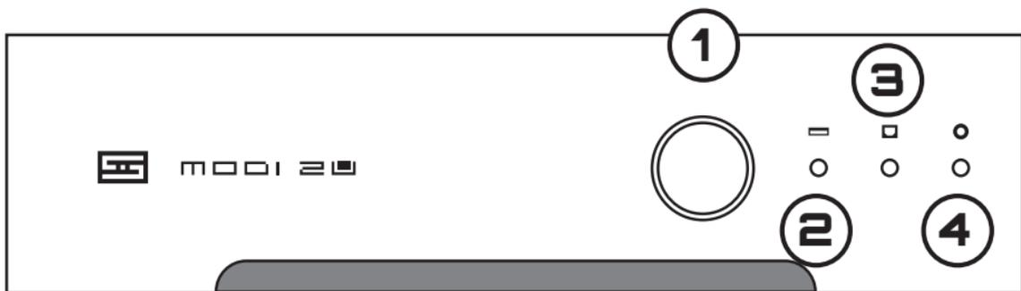
**1** Press the button to cycle through the three inputs and select the one you want to listen to.
