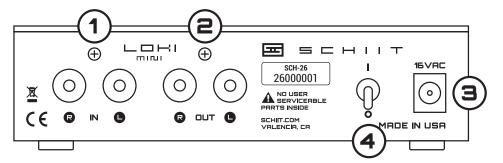
Where to put Loki? You can connect Loki either in-between your source and preamp (if you have a single source) or between the preamp and power amp (so it can be used with all sources.)
