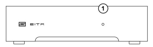
**1 Power Light.** When the power is switched on, this light will illuminate.
