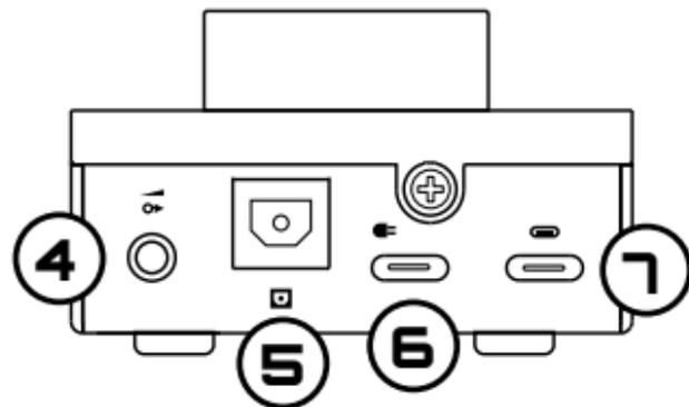
**7 USB Power and Data Input.** Connect this to your computer or other USB source using the provided micro USB cable, or with another USB 2.0-rated, high-quality micro USB cable.
