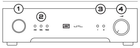
**1 Sample Rate Selector.** Press to step between three different sample rates—48kHz, 96kHz, or 192kHz. Jil does not do 44.1kHz multiples.
