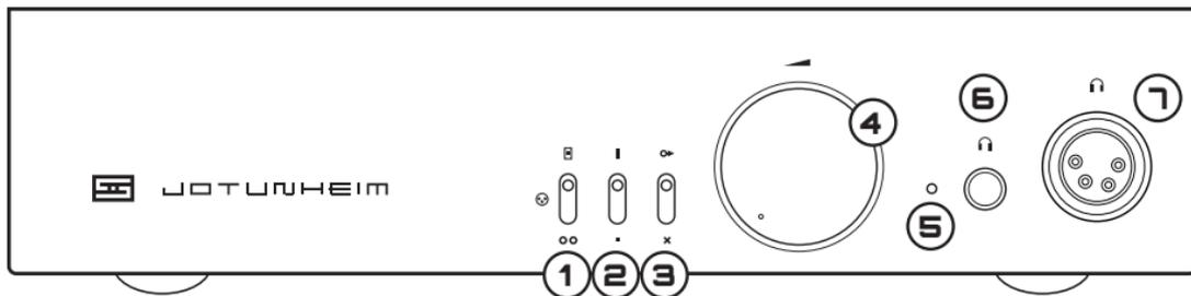
**1 Input Switch.** If the name wasn't clue enough, this selects the input. All the way up for the internal card (DAC or phono), middle for balanced input, bottom for SE input. Hint: if you don't have a card installed, you won't hear anything when the card is selected.
