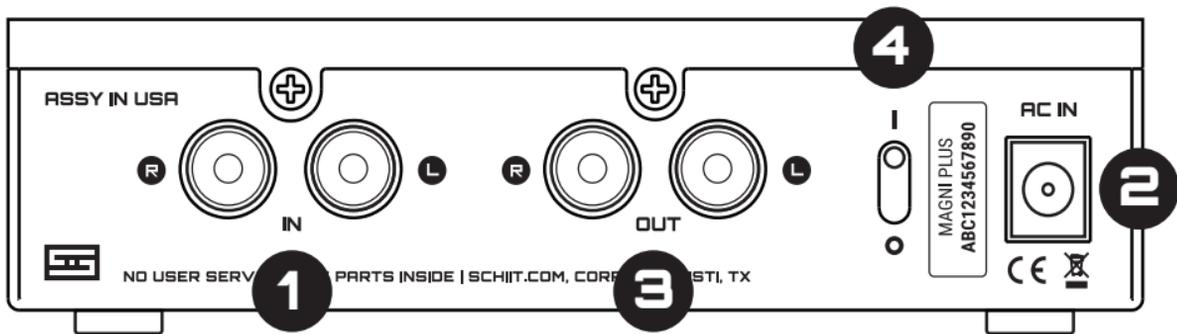
**1 Connect your source to the Magni's "IN" RCA jacks with high-quality RCA cables.** "Source" is a fancy word for DAC, phono preamp, or any other device that has audio output on RCA jacks.
