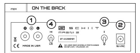
1 Connect your source to the Magni 2's RCA jacks, labeled "L" and "R" with high-quality RCA cables. Alternately, you can use crappy cables if you really want to.
