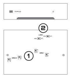
There are no controls on the front, just a LED. When the light is on, it's on. Flip Mani over and you'll see a bunch of switches.
