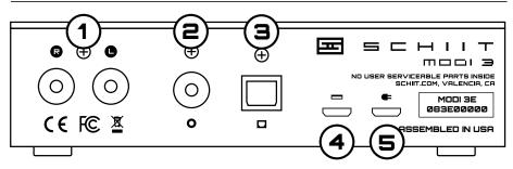
**1 RCA Analog Outputs.** Connect the two RCA jacks, to your amp, preamp, or receiver.
