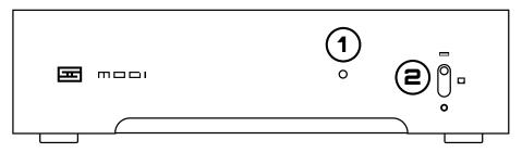
**1 Power LED.** This lights up when you have Modi 3E plugged into a computer, or into an external power source. It doesn't signal UFOs or anything.
