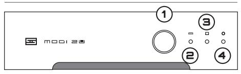
**1** Press the button to cycle through the three inputs and select the one you want to listen to.
